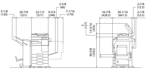
Main unit + DF-633 + PC-218 + FS-539 SD + RU-514 + MK-748 + CU-101 Unit: inch (mm)
