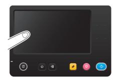
• On the **Control Panel**, press the **Power** key. If the Weekly Timer setting has put the machine in Erp Auto Power off mode, press the **Power** key to display the **Touch Panel**. To use it outside the preset operating hours, follow the on-screen instructions.
