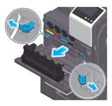
**3** Remove the **Printhead Cleaner** from the **Front Door** of this machine.
