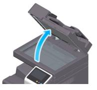
2 Wipe stains off the **Slit Scan Glass** using a dry, clean cloth.
